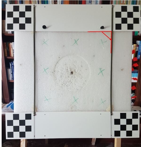
Chessboard plates on target, the required right angle marked in red
